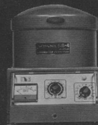
SS-4 MANUAL SUPERSPEED CENTRIFUGE RCF's to 34,800 x g • Speeds to 17,000 rpm • The modern manually-controlled centrifuge; with Gyro-Action Drive!
