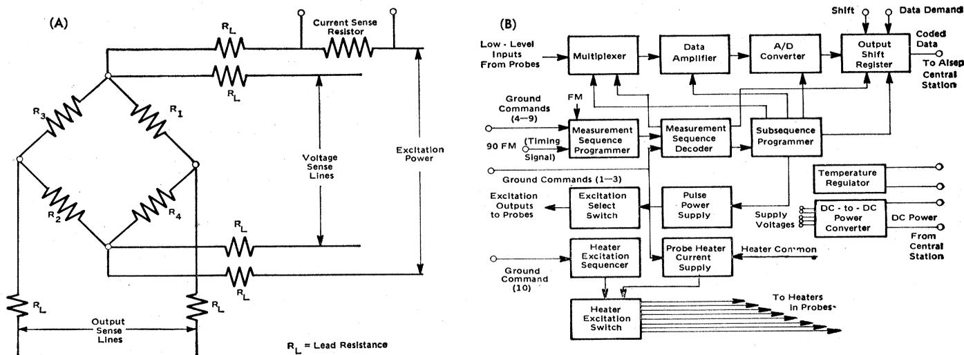
Fig. 5. Schematics of the heat flow experiment measurement system. (A) Configuration of gradient and ring sensor bridges. All bridge resistive elements are platinum wires that are interconnected with Evanohm wire. (B) Block diagram of the heat flow experiment electronics system. The circuitry is contained in a thermally controlled box on the lunar surface separate from the ALSEP central station.
