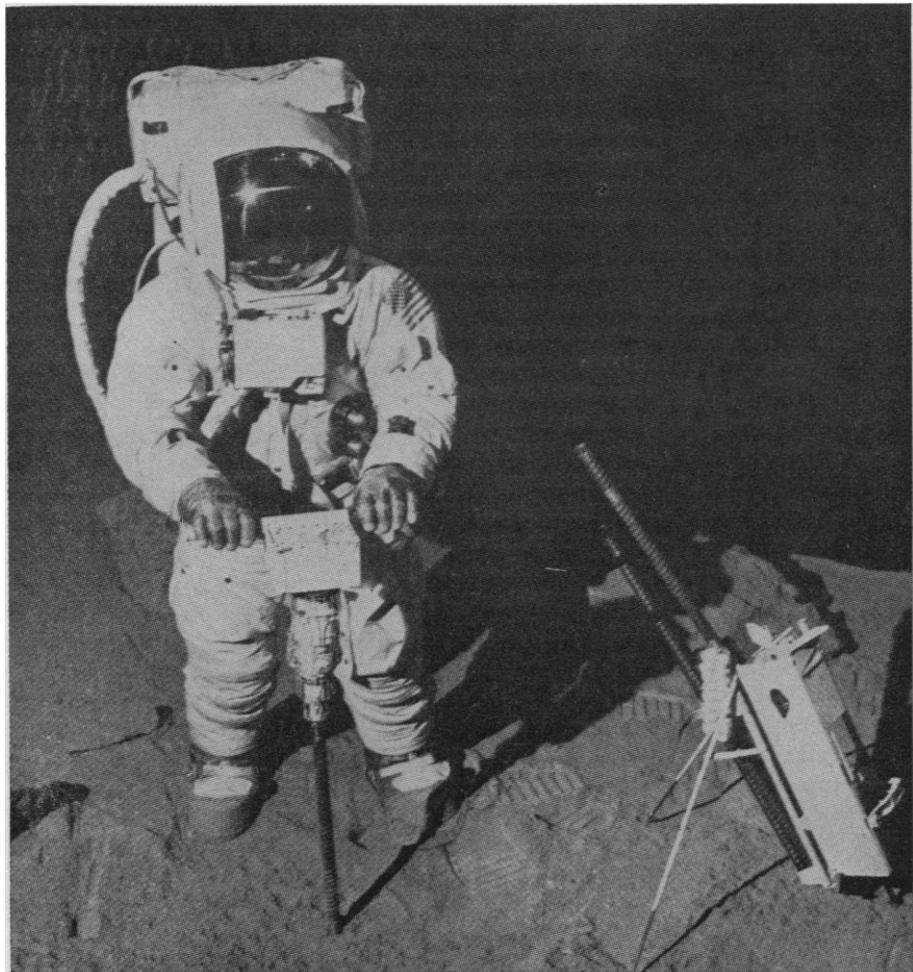
Fig. 2. The lunar surface drill during space-suited tests at the Martin Marietta Corporation. A  $\frac{1}{2}$ -horsepower electric motor in the power head delivers rotary and percussive energy to the drill stem. The motor is powered by silver-zinc batteries with a capacity of 300 watt-hours at 24 volts. The drill rod used to make the heat flow holes consists of interconnecting sections, each 50 centimeters long, of tubular fiberglass reinforced with boron filaments.
