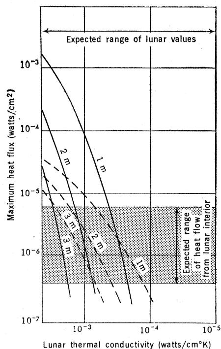
Fig. 3. The maximum amplitude of the periodic heat flow induced by the lunation and annual cycle at 1, 2, and 3 meters below the surface of the regolith is shown as a function of thermal conductivity. Solid line, diurnal wave (first harmonic); dashed line, annual wave. Numbers on curves represent depth below surface.
