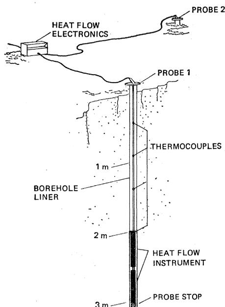
Fig. 1. The heat flow experiment as it may appear in the lunar surface.
