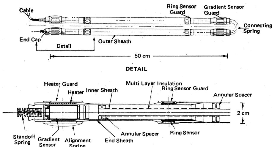
Fig. 4. (Top) The heat flow probe, which consists of two tandem 50-centimeter sections, is shown with the sections folded as they are in their flight package. (Bottom) A detailed drawing of one end of a probe section shows the arrangement of sensors and heaters.
