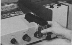
1. Press sample vessel up against Autofill intake trigger.
