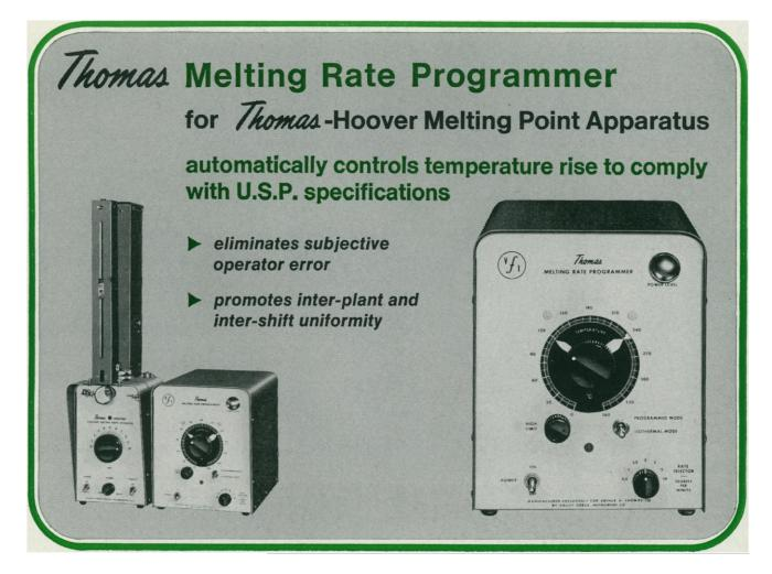
For automatically controlling rate of temperature rise in Thomas-Hoover Melting Point Apparatus. Ensures compliance with U.S.P. specifications for melting point determination on pharmaceutical products. Increases accuracy of m.p. determinations by eliminating subjective operator error in establishing and maintaining constant melting rate.
