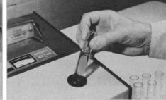
8. Remove cuvette from spectrophotometer.
