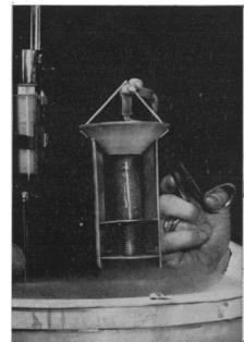
Small quantities of blood are instantly frozen for long-term storage in the droplet freezer. A mechanically vibrated syringe releases droplets into a revolving drum of liquid nitrogen. The frozen droplets are collected in the base. Thousands of droplets can be collected from each sample for use as reference specimens.
