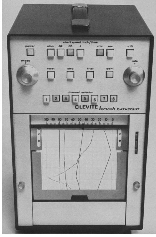
This new high-speed multipoint recorder by Brush runs off as many as 20 samples per second on 2 to 8 patients. So it's great for monitoring fast-changing variables in systemic and wound temperature, heart rate, ECG and the like.
