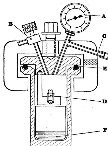
Fig. 1. Sealed cylinder used for the incubation of slices under high oxygen pressure. A, Manometer; B, valve; C, valve of car-tire, for gas entry; D, paper saturated with KOH; E, rubber rim; F, saline (5 ml) in a polythene container. Total volume of the sealed cylinder is 200 ml.
