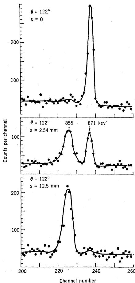
Fig. 4. Gamma-ray spectra indicating the relative change in intensity of the 871- and 855-keV peaks as a function of plunger-to-target distance  $s$ .
