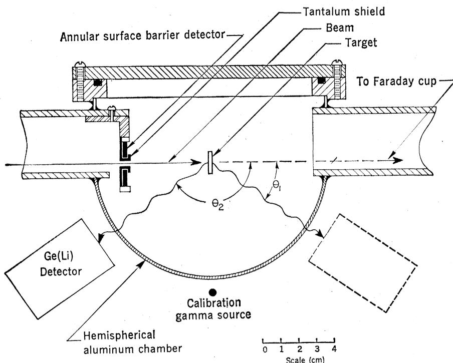
Fig. 7. Experimental arrangement used by groups at Oxford and Rutgers universities to measure lifetimes through excitation of states by inelastic scattering reactions. Gamma rays are observed at forward and backward angles in coincidence with particles backscattered into an annular particle detector.
