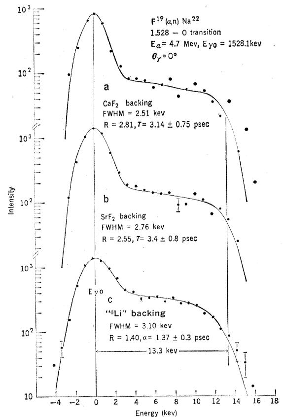
measured line shape and known lifetime. This procedure facilitated the use of  ${}^6\text{Li}$  as a backing in other experiments where the long slowing-down time led to increased experimental accuracy. This case demonstrates the caution that must be taken in these measurements, for a single determination of the lifetime with a backing assumed to be pure  ${}^6\text{Li}$  metal and with  $\alpha=2.1$  picoseconds would clearly give an incorrect result.
