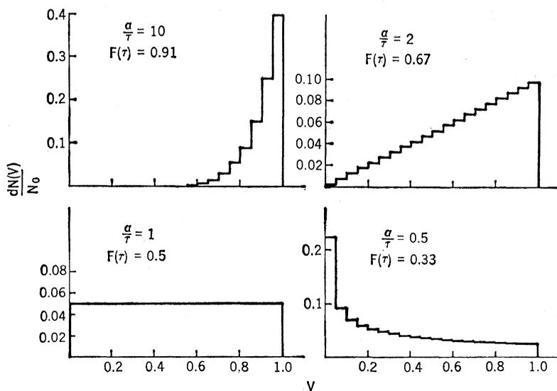
Fig. 10 (above). Theoretical line shapes for various ratios of stopping time to mean lifetime based on the assumption that electronic stopping is the only stopping mechanism.
