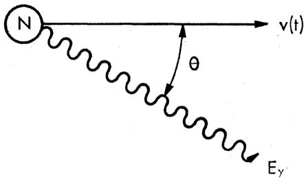
Fig. 1. Schematic diagram of a nucleus moving with velocity  $v(t)$  and emitting a gamma ray at angle  $\theta$  relative to its direction of motion.
