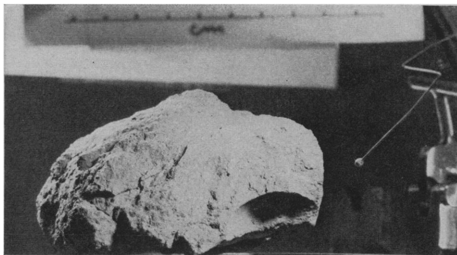
Fig. 2. Sample 12009. This rock, along with sample 12015, displays several large (up to 8 cm) egg-shaped, smooth-walled vesicles. The walls of these vesicles consist of a matte of plagioclase and pyroxene crystals. Rock 12015 is highly shocked, containing about 80 percent glass. NASA photo S-69-62300.
