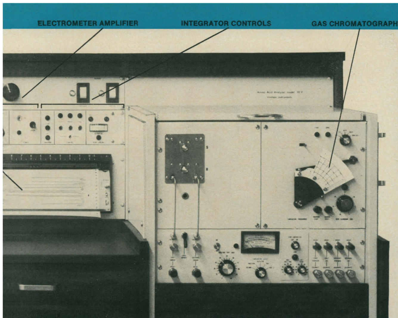
VIVONEX AMINO ACID ANALYZER, MODEL 10V—72 ins. wide by 30 ins. deep by 50 ins. high at the back.
