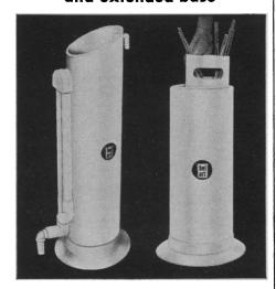
Thoroughly redesigned polyethylene pipette rinser has high level water entry which eliminates the possibility of contaminated water being syphoned back into the public system.
