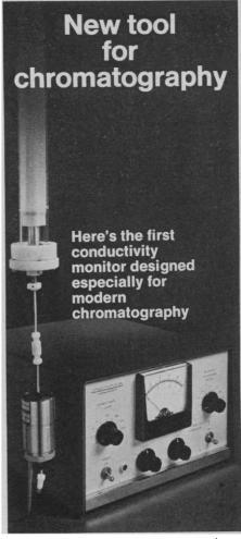
This new monitor detects conductivity as low as .001  $\mu$ mho (.01 ppm NaCl) using a flow-through cell with only 1.5 microliters volume. Response is linear at the recorder output over a million-to-one range from .001 to 1000  $\mu$ mhos.
