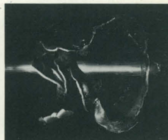
Tensile fracture of copper wire (positive). Type 55 Positive/Negative film.
