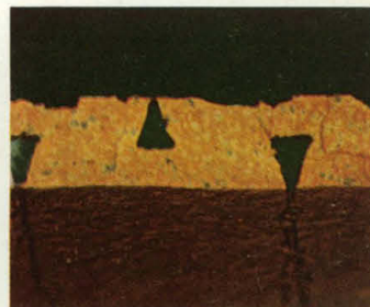
Macro photograph section of battery grid. Polacolor Type 58 film.
