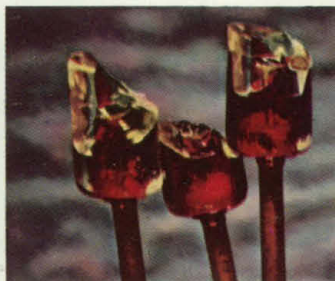
Diode fractures, for QC report. Polacolor Type 108 film.
