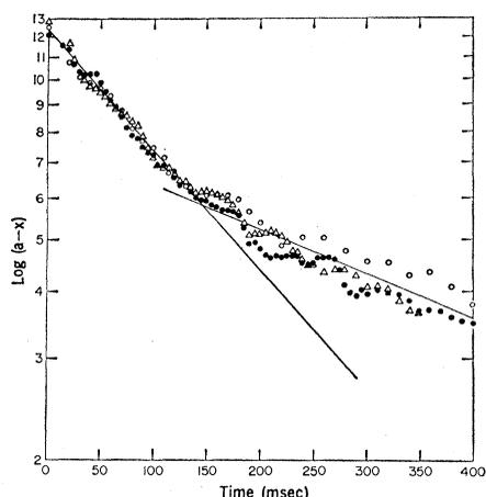
Fig. 3. First-order kinetic plot of the renaturation of acidified nuclease from pH 3.20 to pH 6.70. The value of  $\log(a-x)$  is plotted on the ordinate where  $a$  is the total increase in fluorescence from the beginning to the observed end of the reaction and  $x$  is the increase in fluorescence at any time.
