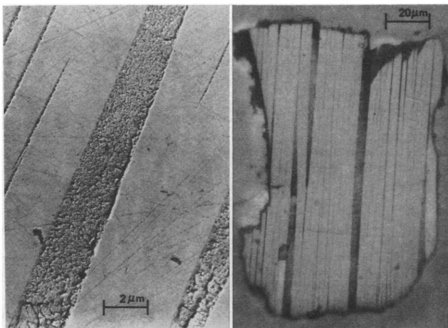
Fig. 1. A pyroxene grain from powder sample 10084,93. The particle composition is: SiO<sub>2</sub>, 53.5 percent; MgO, 18.9 percent; FeO, 27.9 percent; CaO, 2.2 percent (hypersthene).
