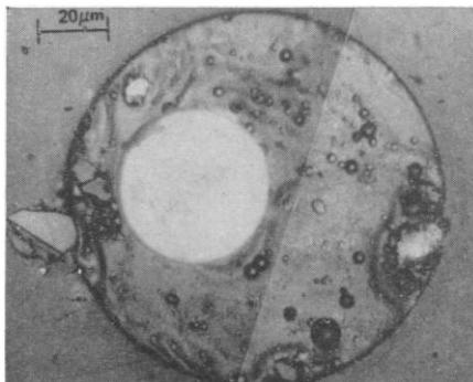
Fig. 2. Lapped and etched section of a glass sphere from powder sample 10084,93. Impact adhesion of small grain on left side is seen with etched interface. The light circle is a spherical cavity.
