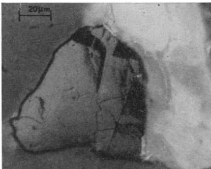
Fig. 3. Photomicrograph of chemically etched pyroxene deformation bands. The heavily etched crystal is a plagioclase.
