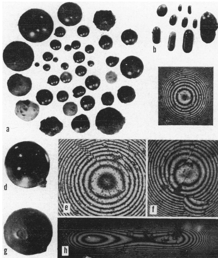
Fig. 1. Photomicrographs of objects found in a sieved sample of lunar dust. (a) Spherules; (b) cylinders; (c) typical fringe pattern in spherical shiny, glassy objects; (d) typical tail-like attachment on a spherule; (e) microcracks in a broken spherical object; (f) microchips in a broken spherical object; (g) a sphere with a small foreign object embedded in its surface; (h) fringe pattern in a typical cylinder.
