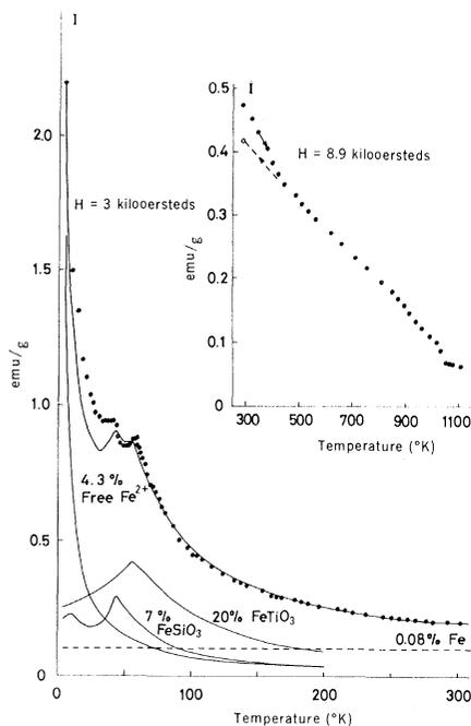
Fig. 1 (left). Magnetization ( $I$ ) versus temperature ( $T$ ) for lunar crystalline rock 10024, 22. Solid circles are observed values; unbroken lines are the simulated curve and the basic curves of the dependences of magnetization of  $\text{Fe}^{2+}$ ,  $\text{FeTiO}_3$  on temperature; the broken line is the basic dependence of the Fe particle on temperature.
