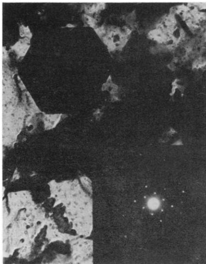
Fig. 3. Electron transmission image and electron diffraction pattern of a hexagonal flake ( $a_0 = 5.15$  Å;  $b_0 = 8.90$  Å) from the lunar soil ( $\times 10,000$ ).
