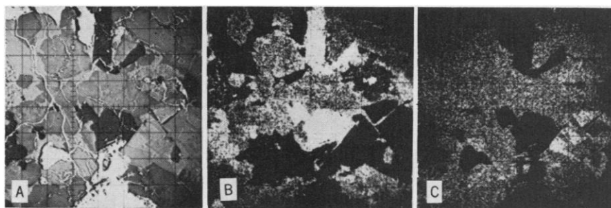
Fig. 2. Electron microprobe scan pictures of sample 10017, type A, showing silica-rich areas mixed with the plagioclase. (A) Target current scan: The darkest areas are ilmenite, the middle-gray areas are pyroxene, and the light-gray areas are plagioclase. (B) Fe K x-ray scan: The brightest areas are the ilmenite, and the next brightest areas are the pyroxene; (C) Si K x-ray scan: The bright areas in the lower right are due to \text{SiO}_2 .
