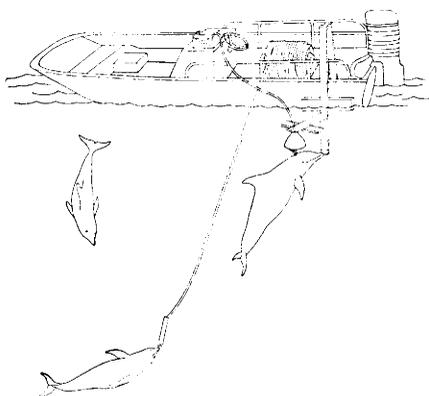
Fig. 1. The experimental setup for deep-diving experiments in the open ocean. The porpoise dives down when the go signal is turned on. He pushes the plunger on the end of the diving test switch, turning the go signal off, and then returns to exhale into the funnel before surfacing.
