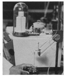
The DP11 is a joy to use. Simply place the burette containing the titrant on the balance pan and carry out your titration. The quantity of titrant you dispense by a remotely controlled pinch valve is continuously displayed on the digital readout panel of the balance.
