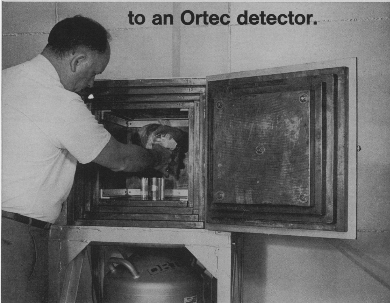
Three-pound container of "lunar fines" goes into a lead shield in special low-level radiation counting facility of the Lunar Receiving Laboratory in Houston. Detector is mounted in the cryostat column, 5 mm from the sample.
