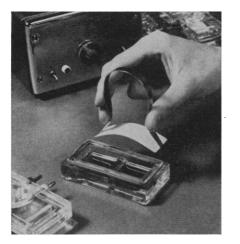
Another feature of the PhoroSlide System is a simple compact and inexpensive electrophoresis cell. No wicks, clips, grips, clamps or tensioning devices are needed to position the
