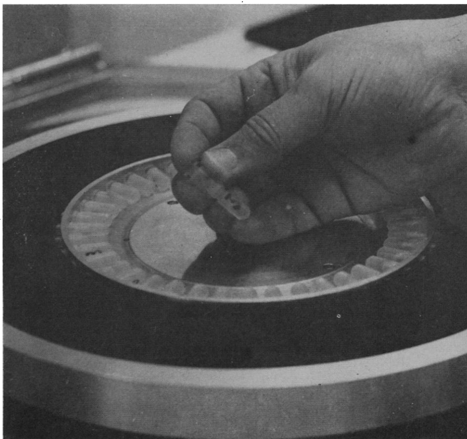
Fig. 7. Small plastic volumetric measuring tubes and transfer disk used to hold tubes during centrifugal transfer of measured liquids into cuvettes (2). Tubes are filled, and the meniscus is flattened centrifugally. They are then placed in the rotor shown and the contents are moved centrifugally into the cuvettes of a cuvette rotor.
