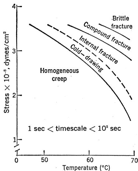
failure of the transparent strip (4) ("brittle fracture," Fig. 2). Specimens that deformed in more than one of the modes described above could also be prepared when stress and temperature were properly chosen (Fig. 1) (4, 5).
