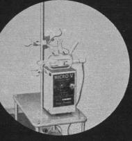
New Clark-type electrode assembly can be used with Gilson Model KM or Model K Oxygraphs without modification. The Clark-type electrode eliminates the problems which occur when using a bare platinum electrode with high protein concentrations and particle suspensions such as whole blood and bacteria, and permits the use of the polarg-graphic method in nonconductive solutions. The response time is only slightly greater than that of the bare platinum electrode.
