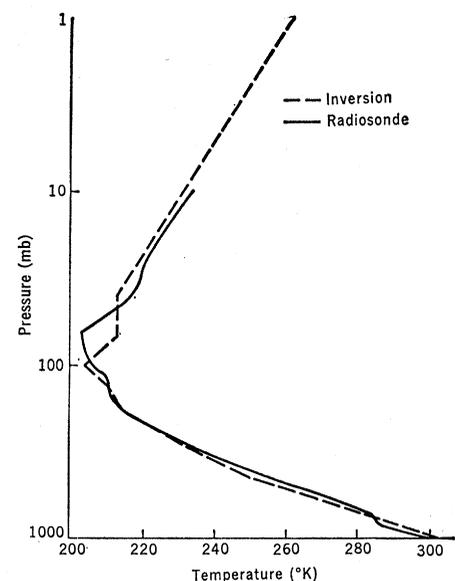
Fig. 2. Temperature profile derived from IRIS data by inversion of the radiative transfer equation; data were recorded near Brownsville, Texas, 22 April 1969 at 1737 G.M.T. Data from a radiosonde ascent at 1800 G.M.T. are shown for comparison.
