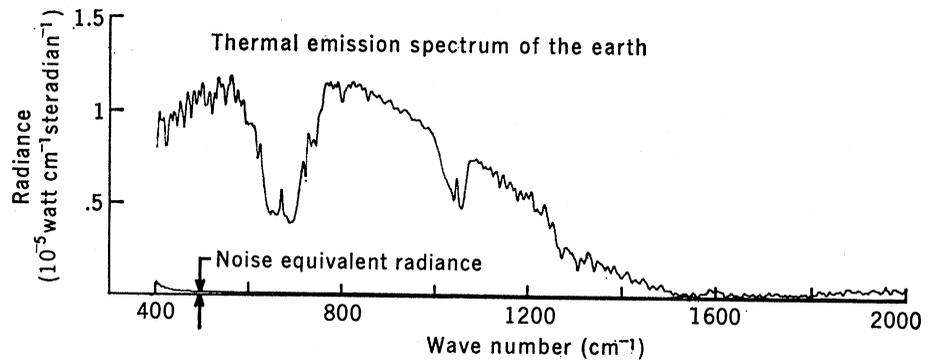
Fig. 1. Thermal emission spectrum of the earth obtained with the infrared interferometer spectrometer (IRIS) carried in the Nimbus 3 satellite. The spectrum was recorded over the equatorial Pacific Ocean on 15 April 1969.
