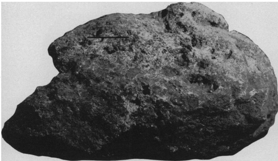
Fig. 10. Photograph of sample 10045 illustrating a type-B rock that displays evidence of original position. The upper-right portion of the sample shows rounding, glass-lined pits, and a light color, whereas the lower-left part of the sample shows sharp angular outline, few pits, and a dark color. It appears that this sample was partially buried on the lunar surface with its upper-left part exposed; scale, 1 centimeter [NASA photograph S-69-45585].
