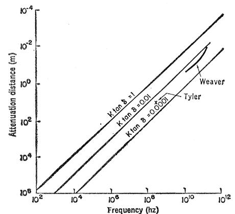
Fig. 2. Theoretical curves for attenuation distance as a function of frequency for constant values of  $K \tan \delta$ . Superimposed values for the lunar surface show that  $K \tan \delta$  is approximately equal to 0.003.
