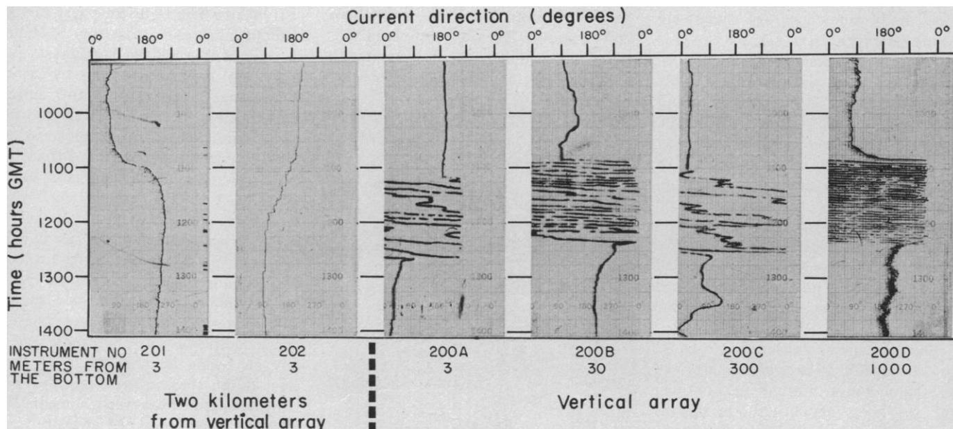
Fig. 4. Records of current measurements just prior to, during, and immediately after the period of the event. The transient event occurred 24 January 1968 at 30°30'N, 119°50'W; depth sea floor, 3950 m (2160 fathoms). (The records for the vertical array were traced on a clear overlay since the original records were too light to photograph.)
