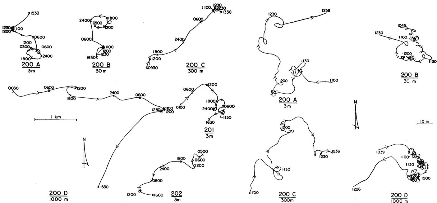
Fig. 2 (left). Vector-addition diagrams for entire record of current measurements. The "event" period is bracketed. Fig. 3 (right). Vector-addition diagrams during the period of the "event."
