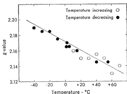
Fig. 2. The effect of temperature on the  $g$  value of the ESR signal exhibited by a pinched frog sciatic nerve. Instrument conditions as described in the legend to Fig. 1.
