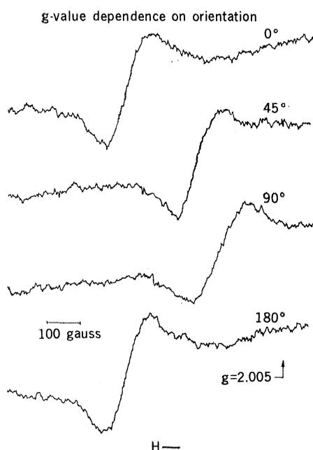
Fig. 3. The angular dependence of the ESR signal from a small segment (about 3 mm on a side) isolated from a pinched nerve. The segment was fastened to the end of a glass rod and inserted into the spectrometer cavity. The rod was rotated on its axis from an arbitrary starting position ( $0^\circ$ ) in  $45^\circ$  steps, and ESR signals were determined in each position. Modulation amplitude, 16 gauss.
