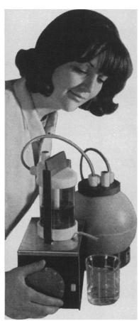
Advanced ultrafiltration systems — with DIAFLO® membranes that retain molecules at levels from 500 to 100,000 MW — can save you hundreds of laboratory hours. Produce up to 1000-fold concentrations of dilute protein solutions without denaturation. Partition complex mixtures or dialyze efficiently and fast even at low salt concentration.
