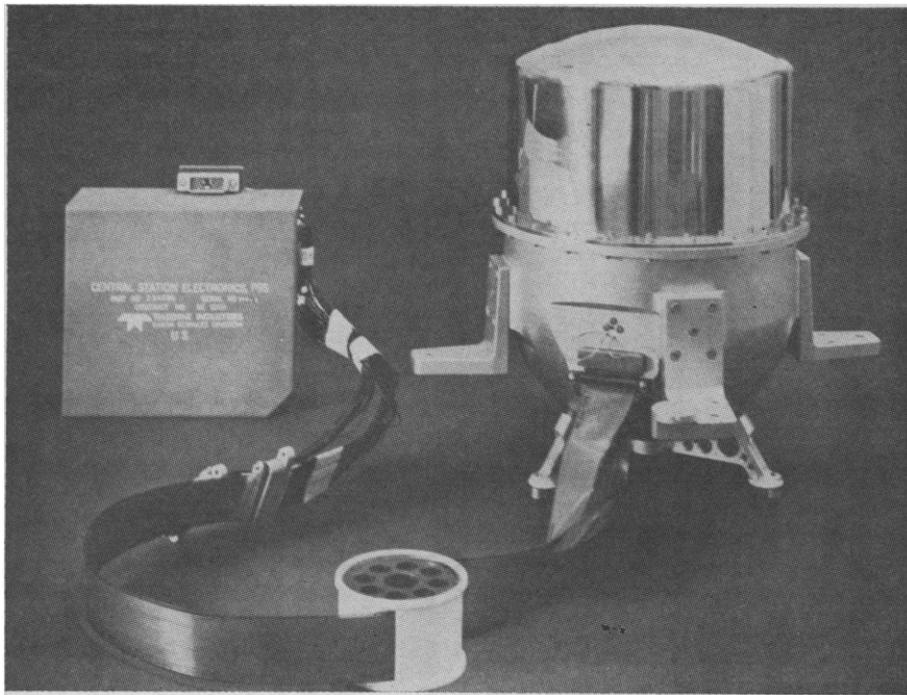
Fig. 5. Photograph of the seismometer system without thermal insulation.
