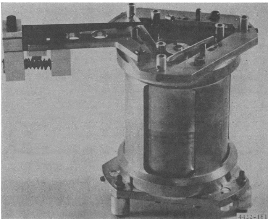
Fig. 8. Photograph of the high-frequency seismometer.
