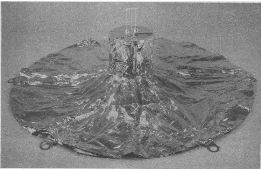
Fig. 6. Photograph of the sensor with the thermal insulation spread out. [Courtesy of the Bendix Corporation]
