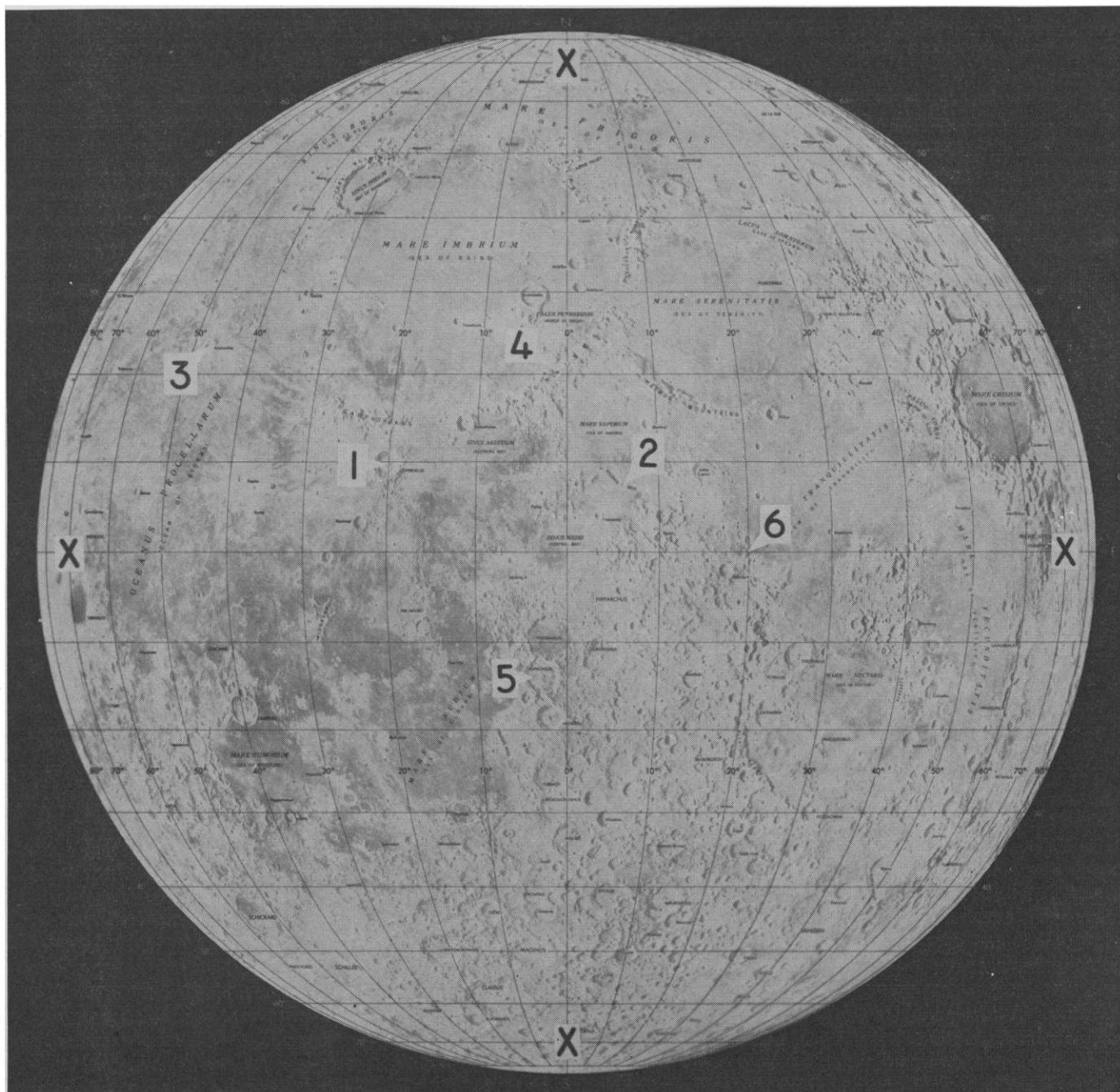
Fig. 12. Suggested locations for an array of lunar seismic stations: (1) floor of Copernicus; (2) Hyginus rill; (3) Aristarchus, floor or surrounding area; (4) Apennine Mountain front; (5) Alphonsus, floor or surrounding area; (6) Sabine and Ritter craters. The X marks indicate sites selected for unmanned lunar landings to complete a lunar seismic net. [From (25), Fig. 3]
