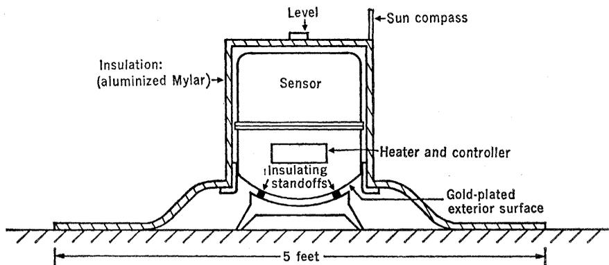
Fig. 2. Schematic diagram of the Apollo passive seismic system.
