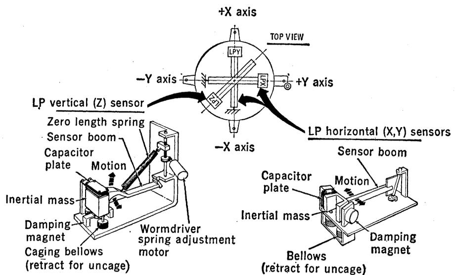
Fig. 4. Schematic diagrams of the low-frequency seismometers. [Courtesy of the Bendix Corporation]
