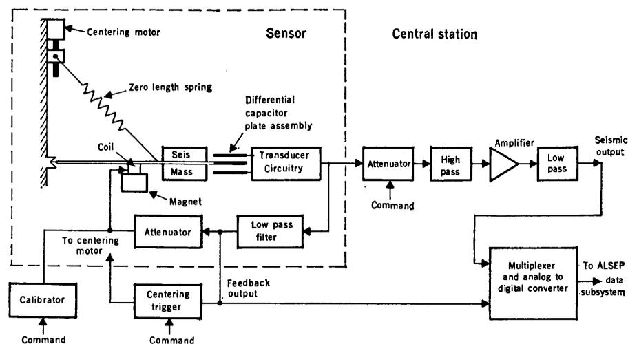
Fig. 7. Schematic diagram of a feedback-controlled seismometer.
