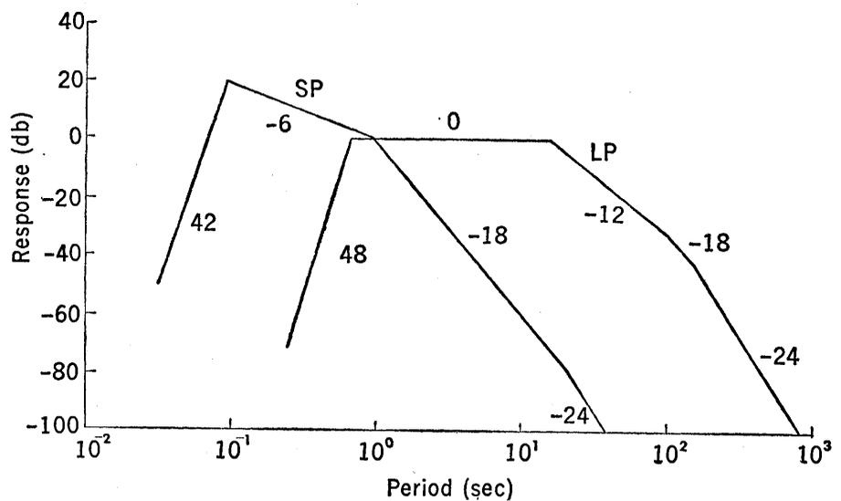
Fig. 3. Nominal response curves of the seismometers; *SP* denotes the short-period seismometer, and *LP* denotes the long-period seismometers. The 0-db level corresponds to a sensitivity of 15 volts per micron of surface motion (maximum gain position).
