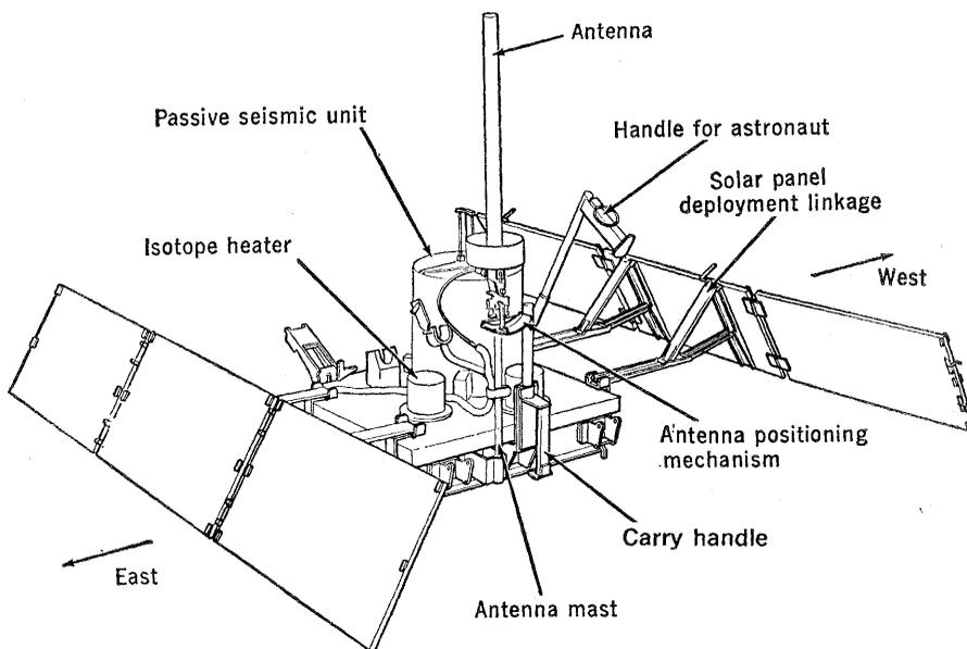
Fig. 1. Passive seismic experiment package (EASEP) as it will appear erected on the lunar surface. [Courtesy of the Bendix Corporation]
