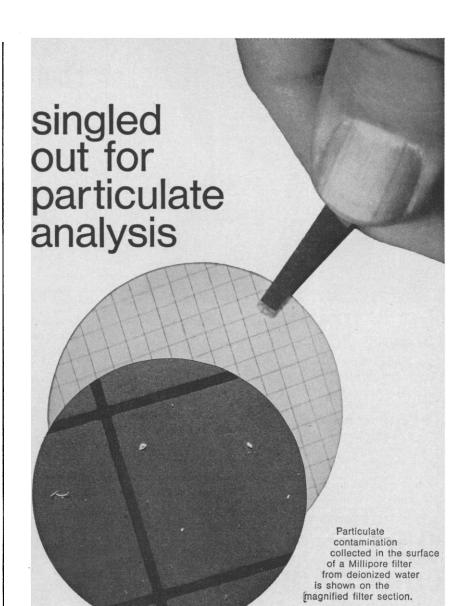
Millipore filters make it possible to isolate micron and submicron particles from fluids and concentrate them for identification and analysis.
