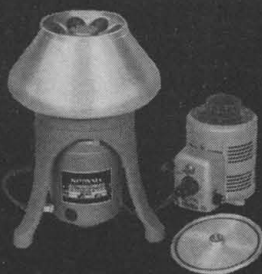
SS-1 SUPERSPEED ANGLE CENTRIFUGE RCF's to 31,000 x G — Speeds to 16,000 RPM. The original "workhorse" of the modern laboratory and still going strong. Adaptable to Continuous Flow Collection.
