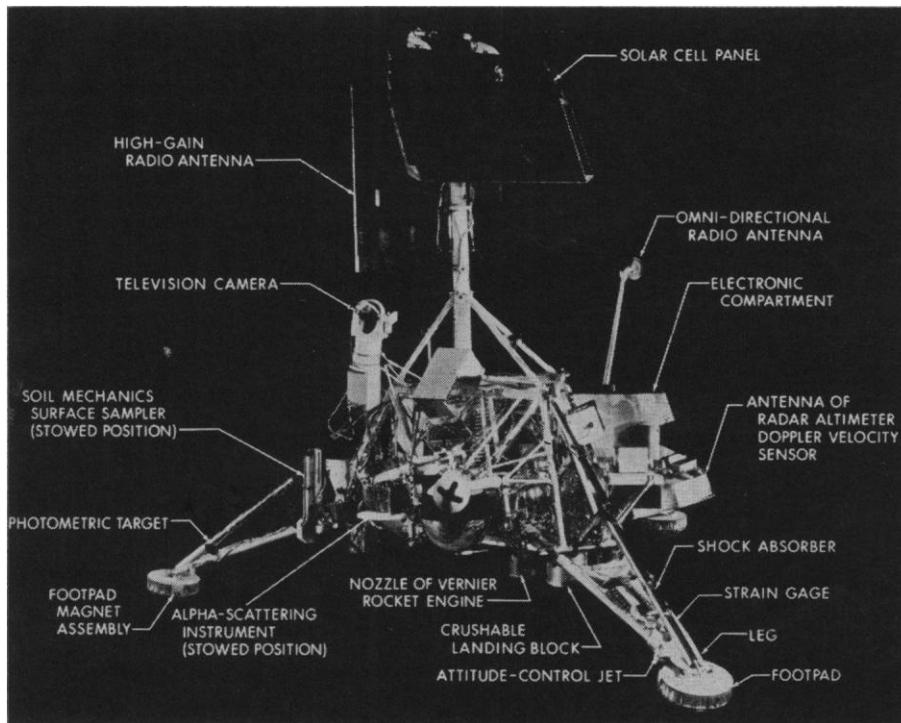
Fig. 2 (top left). Surveyor 7 spacecraft in landed configuration (model).
