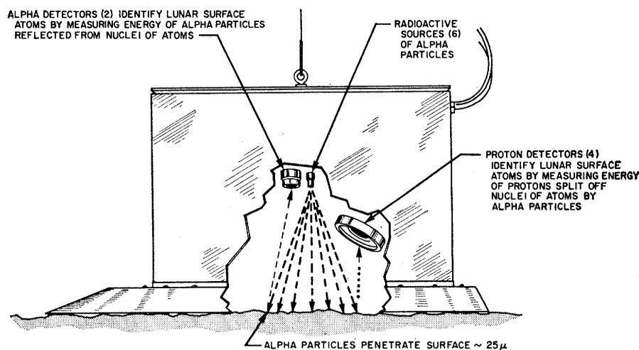
Fig. 5. Surveyor alpha-scattering instrument. View of sensor-head internal configuration. [After Turkevich, Franzgrote, and Patterson (38)]
