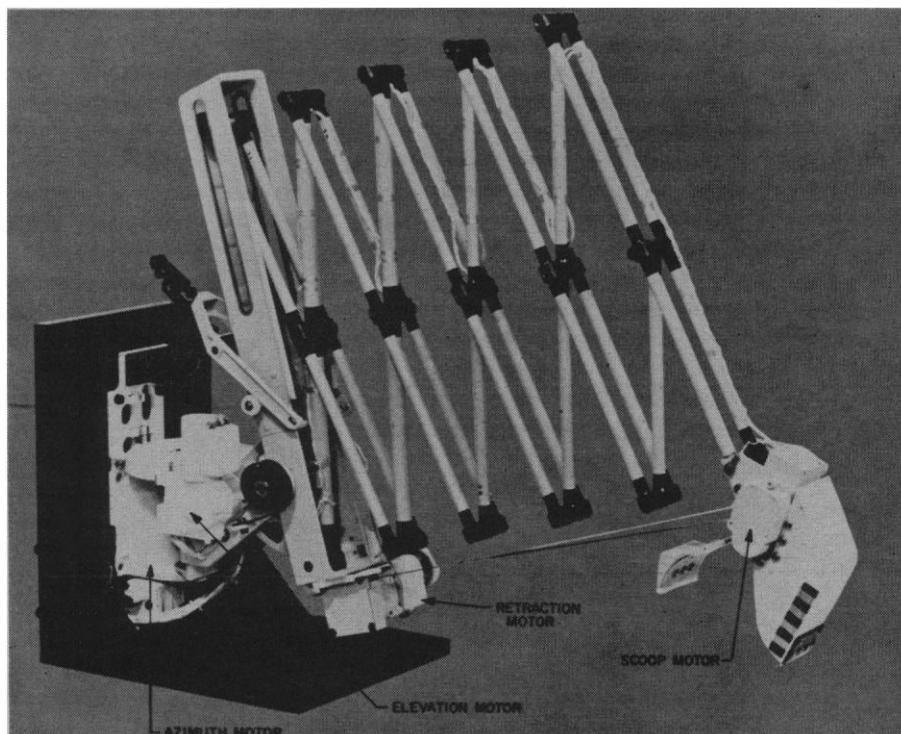
Fig. 4. Surveyor soil mechanics surface sampler.
