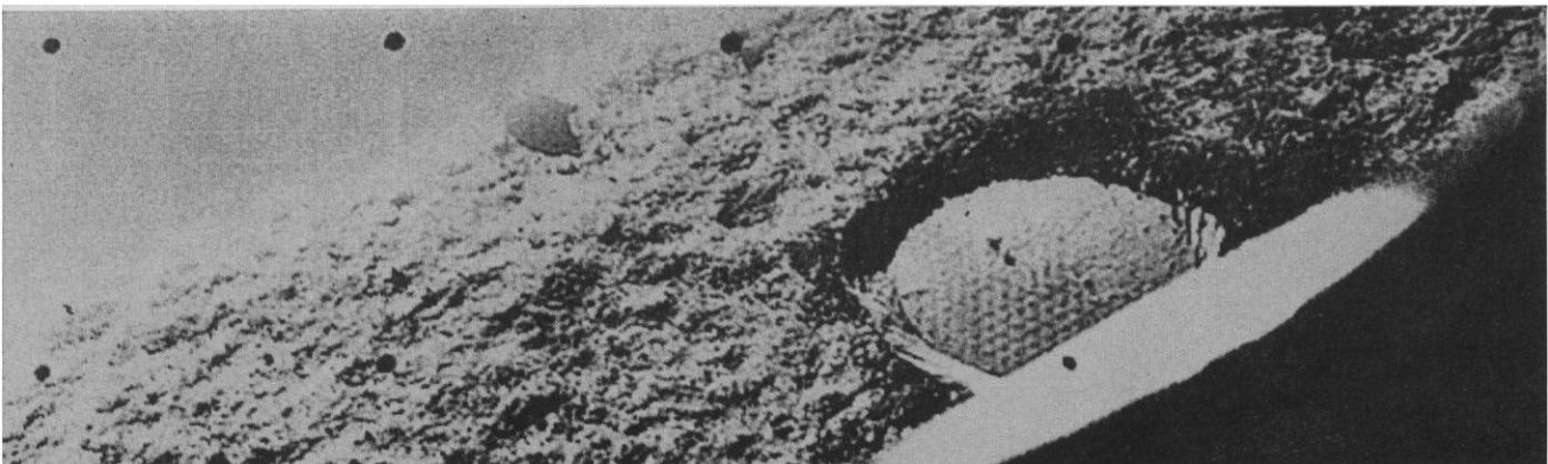
Fig. 19. Imprint on lunar surface of spacecraft footpad. Note replica of waffle pattern on bottom of footpad which had ridges about 60 microns high. (Portion of Surveyor 3 narrow-angle picture taken 21 April 1967, 08:24:20 U.T. Digital computer-processed.)
