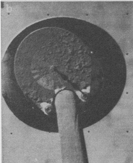
Fig. 16. Lunar material adhering to spacecraft. Photometric target on Surveyor 6 omnidirectional antenna boom (a) before, and (b) after hop. Clod of lunar material was thrown against target by vernier engine exhaust and adhered through landing acceleration of at least  $45 \text{ m/sec}^2$ . Thickness of adhering material is at least 0.9 millimeter. (Narrow-angle pictures taken 17 November 1967, 09:37:05 and 12:30:00 U.T.)
