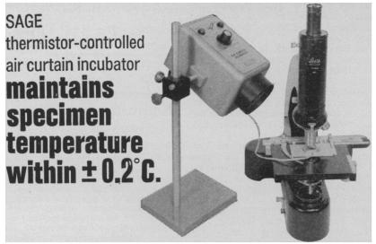
The Sage Air Curtain Incubator controls the temperature of specimens under the microscope within the range of 30° to 40°C with an accuracy of  $\pm$  0.2°C. It totally eliminates the need for enclosures of any kindmicroscope and specimen are completely accessible. Especially useful for biological studies of living materials.
