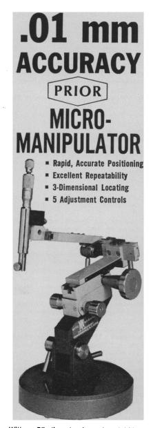
With a 5" diameter base for stability, and a universal rotational height adjustment plus 3 rack-and-pinion gearsets for accuracy, this Prior Micromanipulator is ranked among the finest in hand-operated positioning instruments. Mechanical movements: 64 mm vertical, 28 mm forward horizontal, 65 mm traverse horizontal, tilting traverse 360°; 2 mm vernier in all directions. With micrometer drive, add 13 mm motion with positioning indicated to 0.01 mm. Net weight: 10 lbs.
