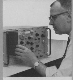
2. Assemble the instrument system you require by plugging the modules selected into a rack-mountable bin which also supplies power to the modules. All Research Instrument Modules are designed to meet the universally-accepted NIM standards developed for modular instruments (AEC TID-20893). These standards greatly simplify assembly of precision measuring systems by providing common power input levels and reducing significantly the need for concern with interface voltages and impedance levels.
