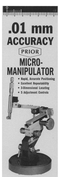
With a 5" diameter base for stability, and a universal rotational height adjustment plus 3 rack-and-pinion gearsets for accuracy, this Prior Micromanipulator is ranked among the finest in handoperated positioning instruments. Mechanical movements: 64 mm vertical, 28 mm forward horizontal, 65 mm traverse horizontal, tilting traverse 360°; 2 mm vernier in all directions. With micrometer drive, add 13 mm motion with positioning indicated to 0.01 mm. Net weight: 10 lbs.
