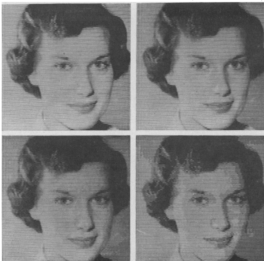
Fig. 2. Early example of computer picture-processing experiments. Various brightness-encoding schemes were tried, and picture quality was assessed. All were displayed on television monitor. (Top left) Original image; (top right) six-bit (64-level) gray-scale result; (bottom left) four-bit (16-level) result; (bottom right) three-bit (8-level) result—too little information preserved for satisfactory representation.
