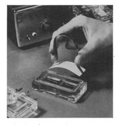
Another feature of the PhoroSlide System is a simple compact and inexpensive electrophoresis cell. No wicks, clips, grips, clamps or tensioning devices are needed to position the springy PhoroSlide strip. As many as ten cells may be connected together for simultaneous parallel operation.
