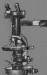
With Binocular Camera Lucida, the first of its kind; up to 1:5 enlargement ratio.
