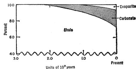
Fig. 2. Calculated present distribution of shale, carbonate, and evaporite as a function of time. The calculation is based on half-mass ages of shale, carbonate, and evaporite of 600, 300, and 200 million years, respectively.
