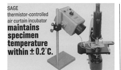
The Sage Air Curtain Incubator controls the temperature of specimens under the microscope within the range of 30° to 40°C with an accuracy of  $\pm 0.2^{\circ}$ C. It totally eliminates the need for enclosures of any kind-microscope and specimen are completely accessible. Especially useful for biological studies of living materials.
