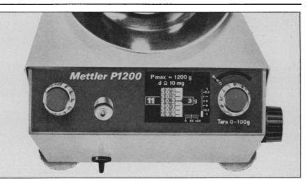
positive reading as weight decreases in drying, evaporation and residue determination studies. This feature eliminates time-consuming calculations and the possibility of arithmetical errors. It also simplifies gravimetric titrations (for more information on the advantages of gravimetric titrimetry, write for Bulletin M-1014A).
