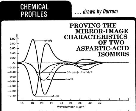
Aspartic acid, with its three donor sites, can form a variety of hard-to-identify chelate isomers. The circular-dichroism profiles drawn here, plotted from data gathered by a Durrum-Jasco CD recorder, are typical of the molecular detective work\* that can be achieved with this versatile instrument.
