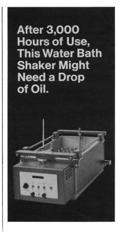
The AO Water Bath Shaker was built to give trouble-free service. And it has in hundreds of laboratories. Sturdy, leak-proof construction features a large volume reservoir made of cast aluminum and coated with Teflon. A ball-bearing eccentric drive and nylon rollers for rack support assure a smooth, quiet shaking action.
