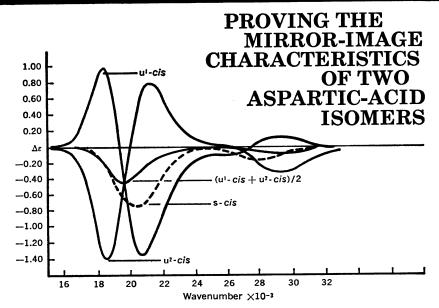
Aspartic acid, with its three donor sites, can form a variety of hard-to-identify chelate isomers. The circular-dichroism profiles drawn here, plotted from data gathered by a Durrum-Jasco CD recorder, are typical of the molecular detective work\* that can be achieved with this versatile instrument.
