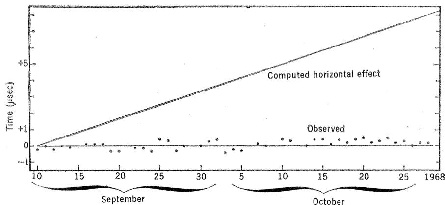
Fig. 2. Difference in times of arrival ( $K$ ) of cycles from Cape Fear, North Carolina, and Dana, Indiana. The quantity plotted is  $(K - 2)$  in microseconds. The difference is  $(100n + K)$   $\mu\text{sec}$ , where  $n$  is some fixed integer.
