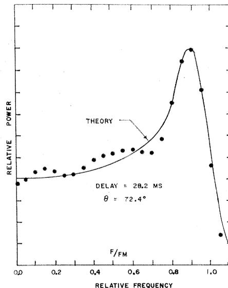
Fig. 2. An averaged spectrum at an incidence angle of  $72.4^\circ$ . The spectrum was folded about the zero-frequency axis to increase the number of independent regions contributing to the spectrum. The observations used were made on 4, 22, and 29 September 1967. Also shown is the least-squares fit of the theoretical spectrum to the observed spectrum points. MS, millisecond.
