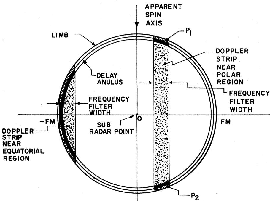
Fig. 1. Delay-Doppler resolution of Venus. Note that all latitudes from the equator to the pole may be observed in a single spectrum if the delay annulus is placed on the limb.  $FM$  is one-half of the limb-to-limb Doppler shift;  $P_1$  and  $P_2$  indicate two regions having the same delay and Doppler frequencies.
