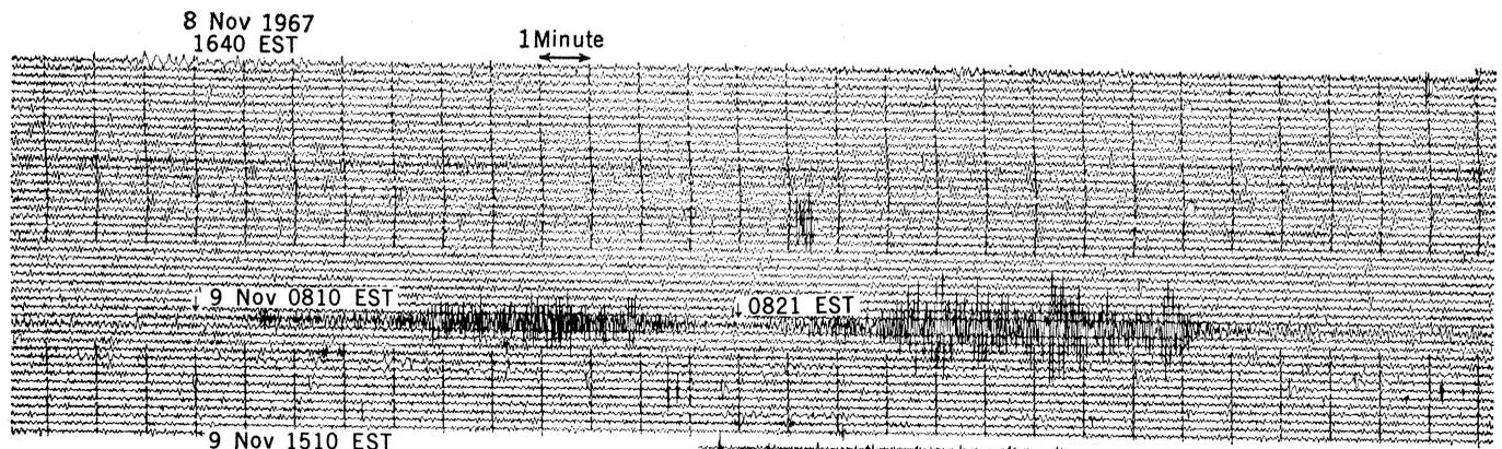
Fig. 2. Capacitor-microphone record of 8 to 9 November 1967, showing the Saturn V infrasound signal beginning about 08:10:30 EST. Time marks are recorded at 1-minute intervals, with clock failure having occurred for a period of 6 hours. Maximum peak-to-peak signal amplitude is about 20  $\mu$ bar.
