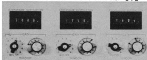
*Model 3320 incorporates Packard's patented arrangement of three completely separate channels of pulse-height analysis, each with precisely adjustable linear amplification and continuously variable discrimination levels. You count each sample only once, and collect data in all three channels simultaneously.*
