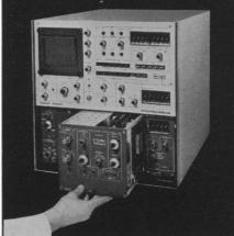
800 & 4000 channel analyzers with plug-in logic for:
