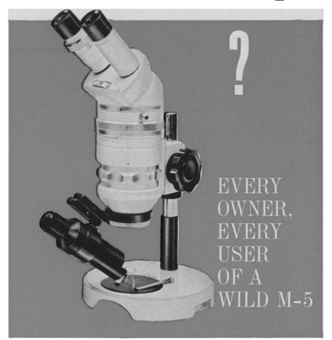
Customer designed power? With easily interchangeable eyepieces and attachment objectives, you can choose the power range you need, from 2x to 200x.
