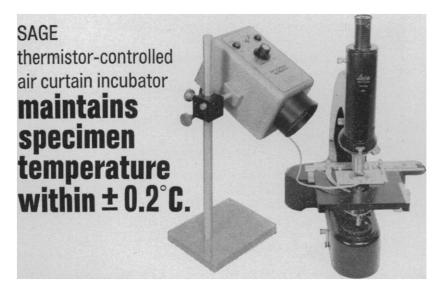
The Sage Air Curtain Incubator controls the temperature of specimens under the microscope within the range of  $30^\circ$  to  $40^\circ C$  with an accuracy of  $\pm\,0.2^\circ C$ . It totally eliminates the need for enclosures of any kind-microscope and specimen are completely accessible. Especially useful for biological studies of living materials.
